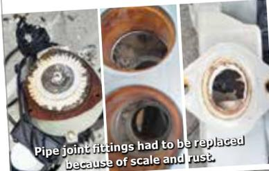
Pipe joint fittings had to be replaced because of scale and rust.
