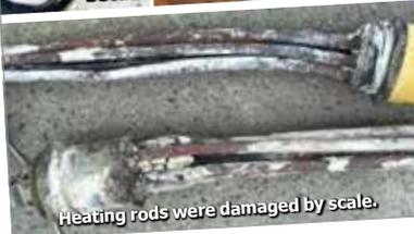
Heating rods were damaged by scale.
